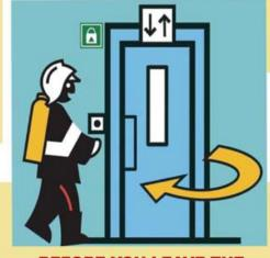
**BEFORE YOU LEAVE THE** INSTALLATION, CHECK THAT ALL **LANDINGS DOORS ARE CLOSED** AND LOCKED.
